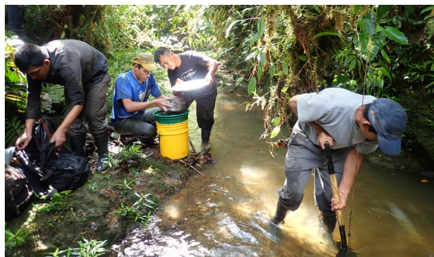
Stream sediment sampling - efficient way of identifying metal enrichment in the area that each stream drains
