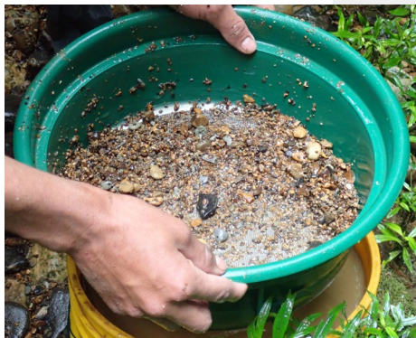
Stream sediment sampling - efficient way of identifying metal enrichment in the area that each stream drains
