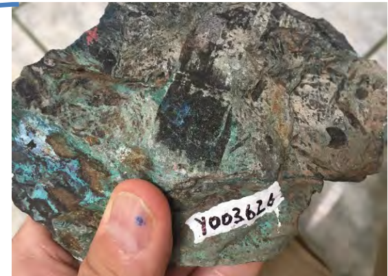
6.4% copper, 48g/t silver in sandstone with carbonized plant fragments
