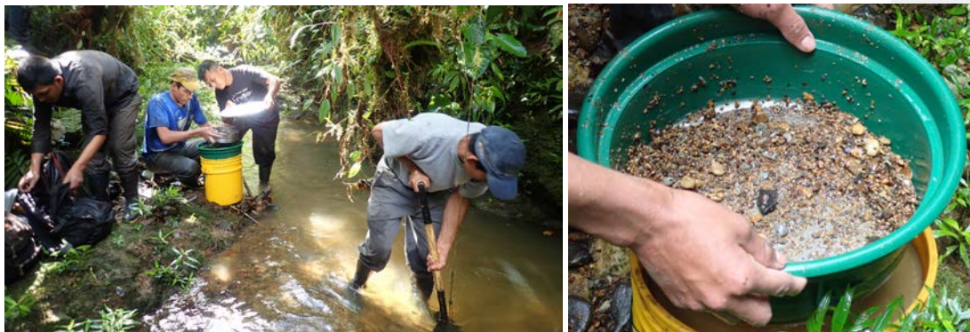
Stream sediment sampling - efficient way of identifying metal enrichment in the area that each stream drains
